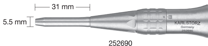
252690 High-Speed Handpiece , extra short, straight, 60,000 rpm, for use with High-Speed Micro-Motor 20 7120 33
