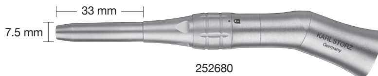
252680 High-Speed Handpiece , short, angled, 100,000 rpm, for use with High-Speed Micro-Motor 20 7120 33
